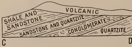
FIG. 163—Geologic sketch section to show the relation of the volcanic flows of Fig. 164 to the sandstones and quartzites beneath.
